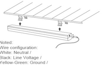
Repeat steps for each fixture length or connect additional fixtures using supplied butt connector or jumper cable.
