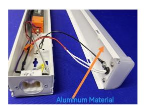
The base holder and aluminum material board can be detachable, so it is convenient to open up for checking or maintenance. Some suppliers do not use the aluminum material, but using the cold rolled steel, so the heat dissipation will be inferior.
