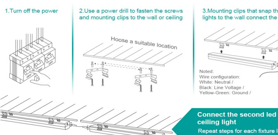
3. Mounting clips that snap the LED lights to the wall connect the AC cable
